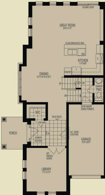
Ground Floor Elevation 'A'
