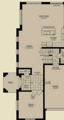
Ground Floor Elevation 'B'
